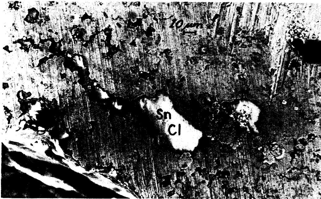
Figure 7. Cross section showing selective corrosion of gamma-2 phase. The cavities are filled with corrosion products containing tin and chlorine atoms. Case B.
