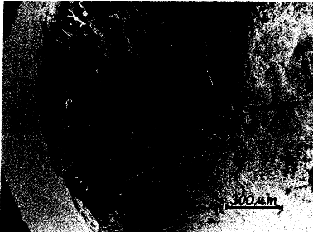
Figure 1. Crevice corrosion of a five year old amalgam filling. Bright area is the buccal surface. Case A.
