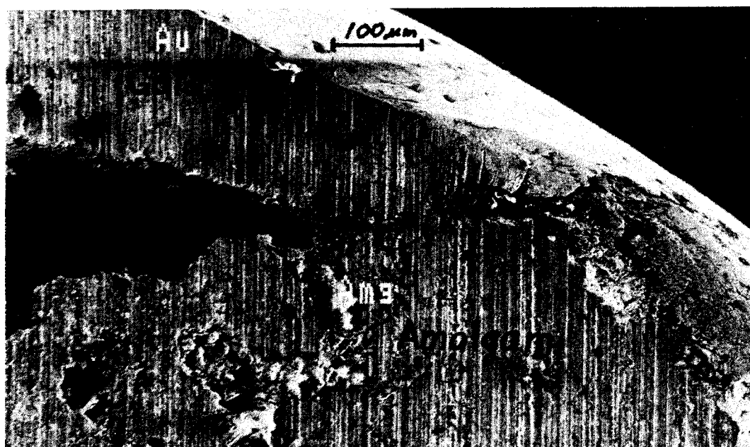
Figure 10. Galvanic corrosion of silveramalgam (Amg) under a gold crown (Au). Case B.
